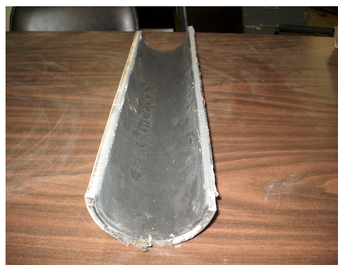
Figure 2.1 and 2.2: Injection pipeline before (thick layer of hydrocarbons/solids around the entire pipe) and after chemical soak & water wash.
