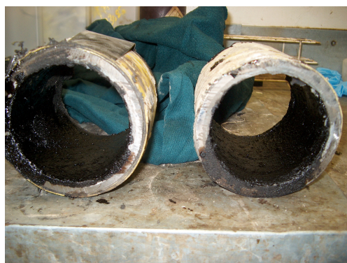
Figure 2.1 and 2.2: Injection pipeline before (thick layer of hydrocarbons/solids around the entire pipe) and after chemical soak & water wash.
